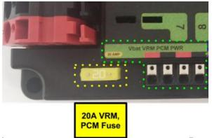
Either of the left two pairs of Weidmuller (red/black) can be used for VRM power. Red is for positive, black is for ground.
