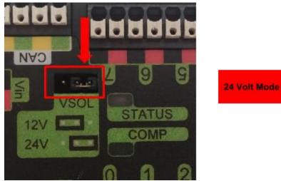
The absence of a Solenoid Voltage Jumper will place the PCM in 24 Volt Mode by default.
